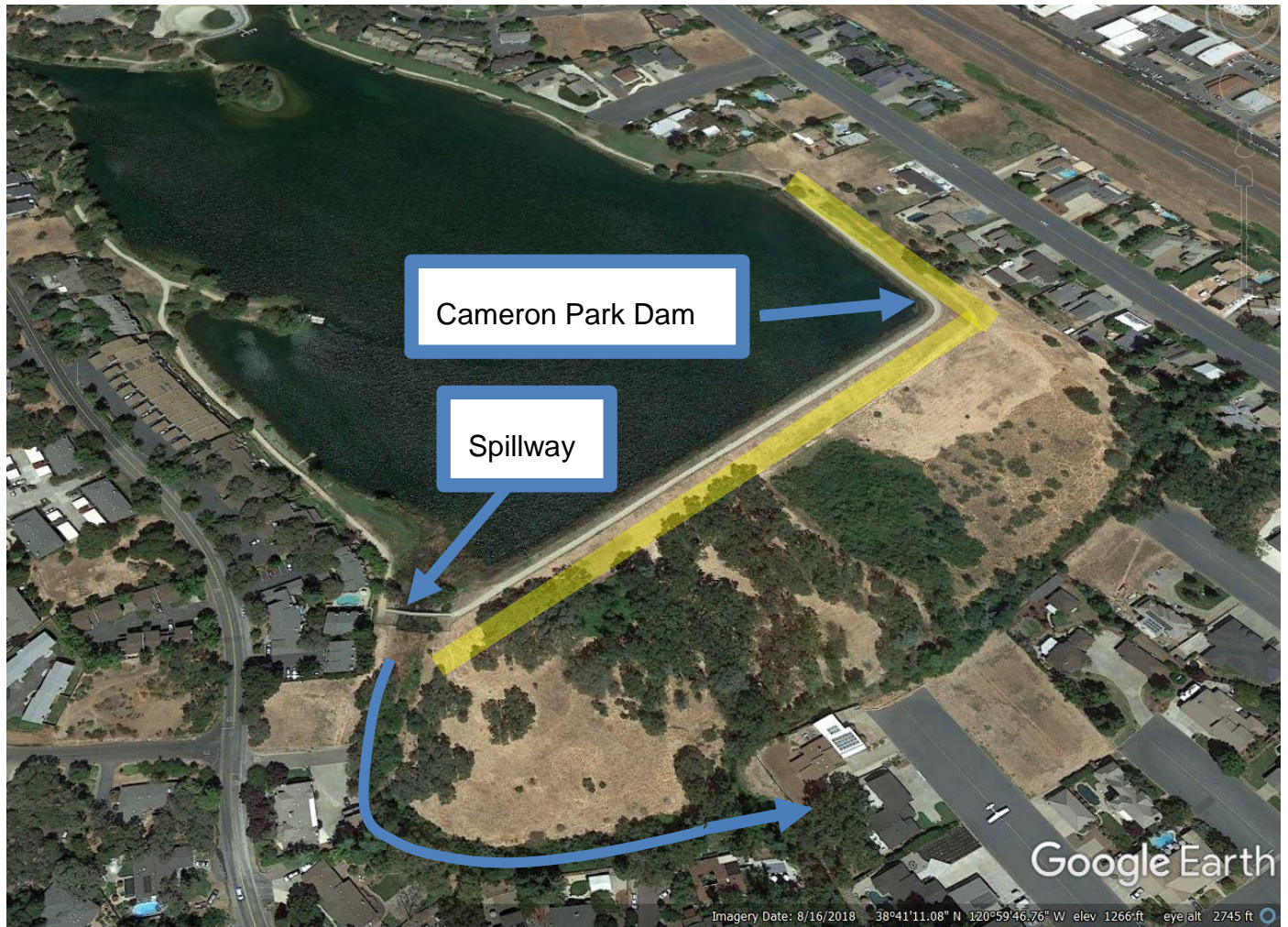
Figure 2. Schematic of Cameron Park Dam and Spillway
